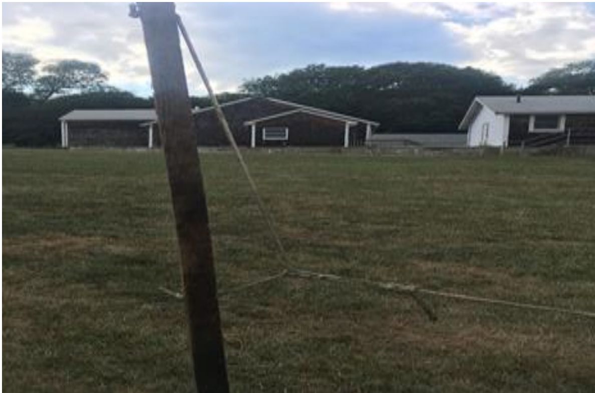
Figure 6. Modified stake allowing the trap to have 2 feet of vertical movement with the tides.
