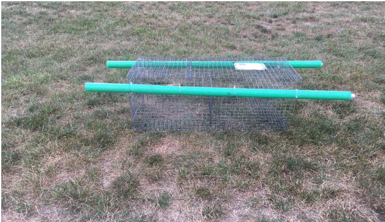
Figure 2. Modified metal box trap with polyethylene foam pool noodles for trap floatation.
